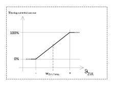
= Temperaturfühler Zuluft  $\theta_{ZUL}$ = Sollwert Zulufttemperatur WZUL-Temp. = Stellsignal Regler Sommer
