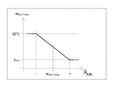
$\begin{array}{ll} \vartheta_{ABL} & = Temperaturf \ddot{u} hler \ Abluft \\ w_{ZUL\text{-Temp}}. & = Sollwert \ Temperatur \ Zuluft \\ w_{ABL\text{-Temp}} & = Sollwert \ Temperatur \ Abluft \end{array}$
