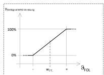
$\begin{array}{ll} 9_{ZUL} & = Temperaturf \ddot{u}hler\ Zuluft \\ 9_{FOL} & = Temperaturf \ddot{u}hler\ Fortluft \\ w_{ZUL-Temp}. & = Sollwert\ Zuluft temperatur \\ w_{2^{\circ}C} & = Sollwert\ Vereisungsschutz \\ y_{Winter} & = Stellsignal\ Regler\ Winter \end{array}$
